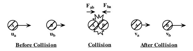
Since two variables are to be determined, the derivation needs two equations. During their collision their total momentum remains equal.
