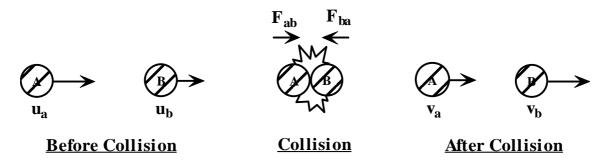
Incase of elastic collision between two bodies A & B, then total kinetic energy should be equal before and after collision. So,
