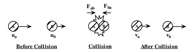
During collision, body B will experience a force  $F_{ab}$  from A in the direction of its motion. So, it will accelerate and thus the velocity changes to some new value  $v_b$  such that  $v_b > u_b$ .
